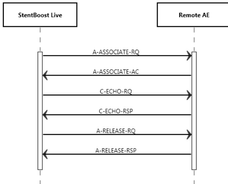
Figure 3: Data Flow Diagram – Verification as SCU
