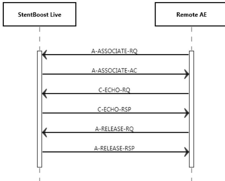
Figure 6: Data Flow Diagram – Verification as SCP
